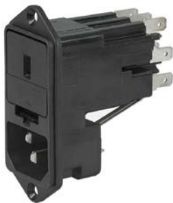
IEC connector C14 with fuse holder 1- or 2-pole Screw-on version from front or rear side with voltage selector
