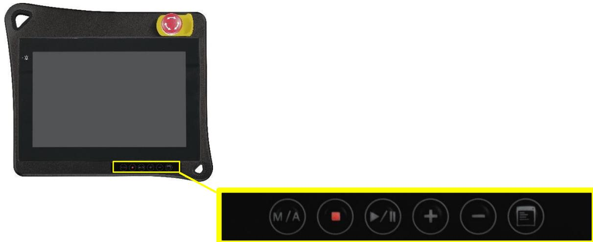
The TP-100-1's membrane keys are located at the lower-right of the teach pendant, each membrane key is mapping to the real-keyboard signal, review the key definitions below:
