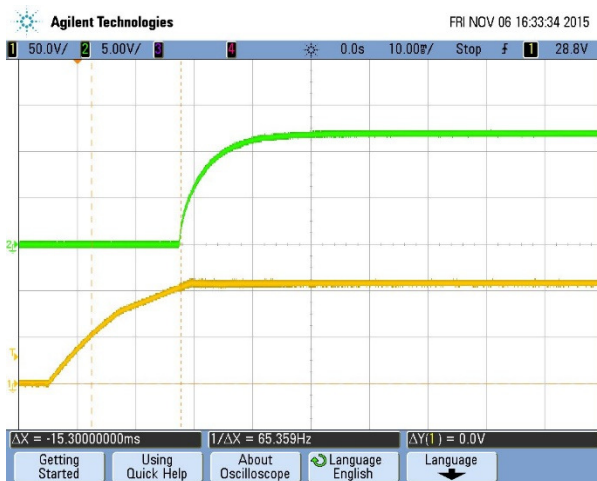
Figure 17: Turn-on transient at zero load current (10 mS/div, Top Trace: Vout, 5V/div; Bottom Trace: Vin, 50V/div)
