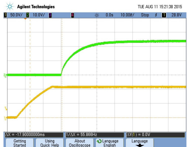
Figure 30: Turn-on transient at full load current (10 mS/div, Top Trace: Vout, 10V/div; Bottom Trace: Vin, 50V/div)
