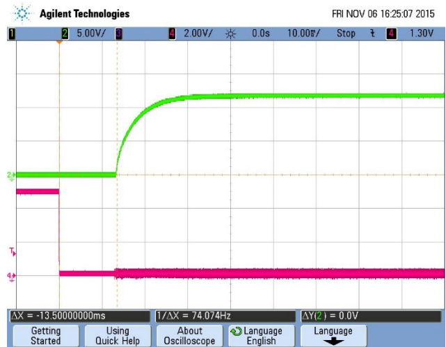
Figure 16: Turn-on transient at full load current (10 mS/div, Top Trace: Vout, 5V/div; Bottom Trace: ON/OFF, 2V/div)
