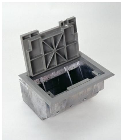
The AF1 Raised Floor and Stage Floor Box provides three separate compartments that accommodate a combination of power, communication and audio/video devices. This combination is accomplished with the built-in service dividers. These dividers are arranged in a single-double, single-gang configuration. Die-cast aluminum housing provides added strength and reliability.
