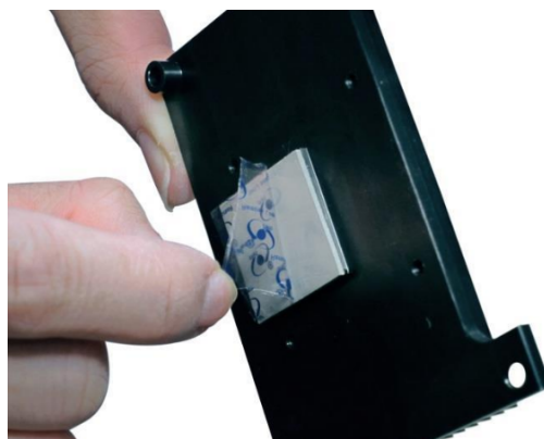
Figure 5: Removing the plastic film from the TIM
