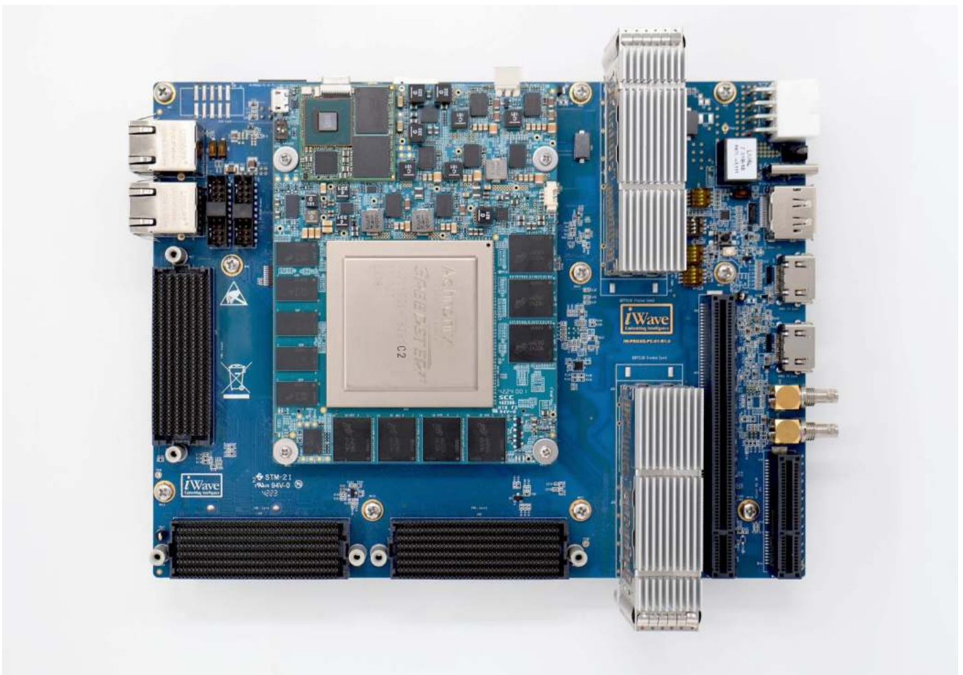
Figure 13 : iW-RainboW-G64D-Speedster7t FPGA SOM Development Platform
