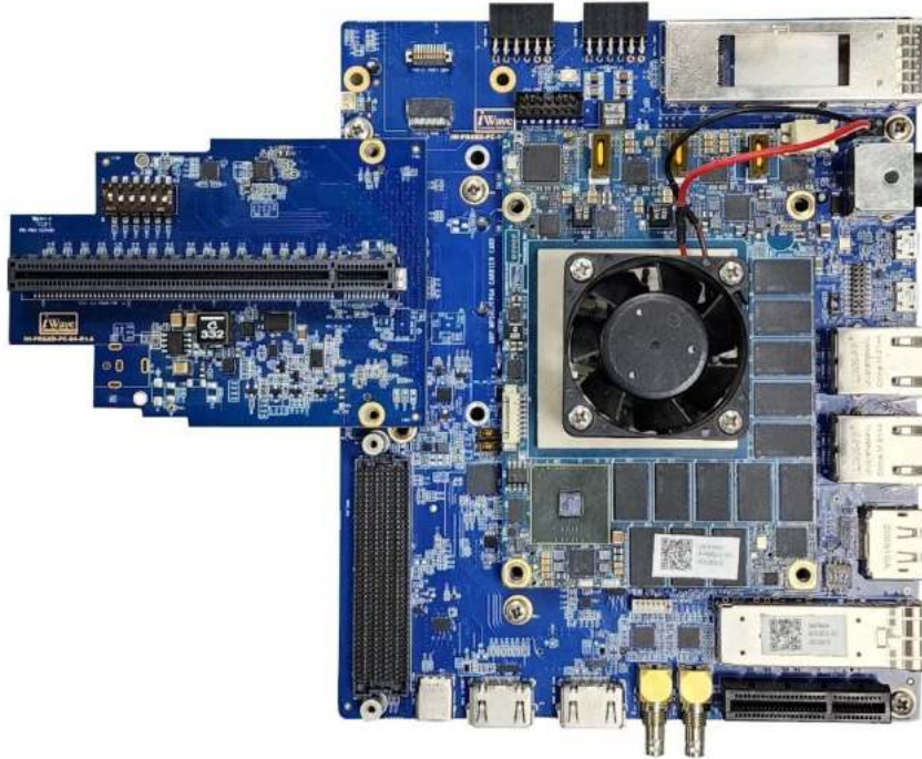
Figure 13: Inserting FMC+ Module in Development Kit
