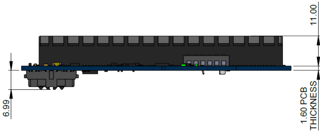
Figure 11: FMC+ PCIe x16 Module Mechanical dimension – Side View
