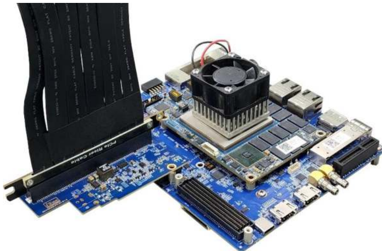
Figure 14: PCIe x16 Cable insertion in FMC+ Module
