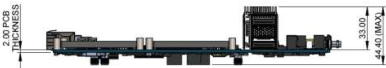
Figure 42: Development board Mechanical dimension – Side View
