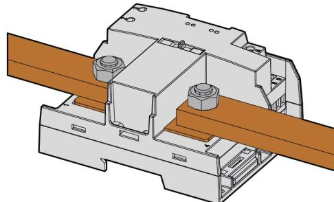
*Fig. 1 Bar-bar mounting*
