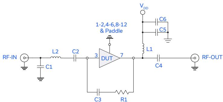
Fig 1. Block Diagram of Test Circuit used for characterization. (DUT soldered on Mini-Circuits Characterization test board TB-1063-13LN+) Gain, Return Loss, Output Power at 1 dB Compression (P1dB), Output IP3 (OIP3) and Noise Figure measured using Agilent's N5242A PNA-X microwave network analyzer.
