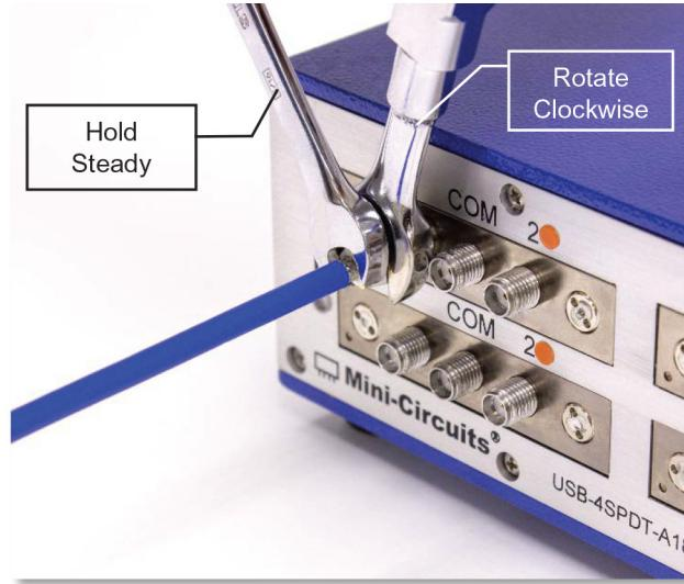
3) Using a 5/16-inch open end wrench, rotate the coupling nut clockwise to tighten the cable connector.
