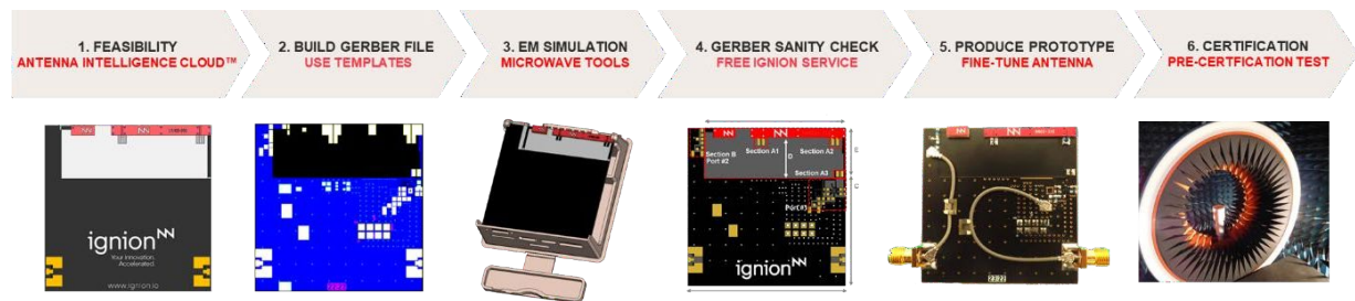
Figure 13 – Virtual Antenna® design journey for a successful IoT solution.
