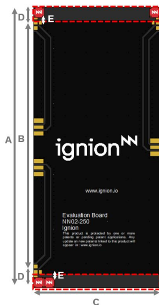
Figure 5 – EB_NN02-250-CPW3R. Evaluation Board with coplanar grounded transmission lines. 698 MHz to 798 MHz, 824 MHz to 960 MHz, and 1710 MHz to 2690 MHz.
