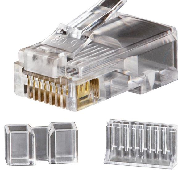
Klein's data and telephone plugs are professional-grade and deliver consistent, reliable performance. Our thick 50 micro-Inch gold plating on contacts prevent erosion and extended connector life. The three-pronged contacts provide more reliable connections with solid and stranded wire. The plug is housed in a durable resin with a spring clip. Expect a sure connection each and every time.
