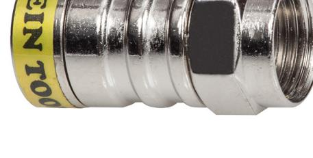
The innovative design of the Klein VDV812-627 Push-On Connector-F allows the cable and connection to reliably turn inside the connector shell, reducing cable strain when packing in a wall box or behind equipment. No tools are necessary for installation. A color-coded application band allows for easy identification of cable compatibility.
