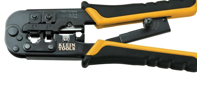
The all-in-one Ratcheting Modular Crimper/Stripper cuts, strips and crimps paired-conductor cables (round STP/UTP and flat-satin phone cables). Durably made from steel and finished in black oxide for high performance, it provides fast, reliable modular-crimp connector installation for voice- and data applications. Crimps 4, 6, and 8 position modular connectors (RJ22, RJ11/RJ12, and RJ45).
