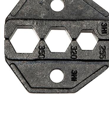
For use with Klein VDV200-010 Replacement Ratcheting Crimping Frame. Designed for Hex Crimp RG59/RG6 Coaxial Cable F-Connectors. Dimensions: 0.255 in. /0.320 in. /0.350 in. Durable construction. Crimp die for use with crimp connectors. Not for use with compression connectors.
