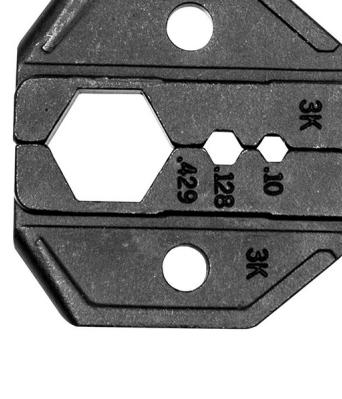
Klein Tools VDV211-043 RG8/11/174/179/213 Coaxial Cable Die Set is for use with Klein's VDV200-010 Replacement Ratcheting Crimping Frame with Hex Crimp Connectors (sold separately). Made from induction hardened high-carbon steel for durability and long life. Designed to be easy to change from one to the next and for multiple uses.
