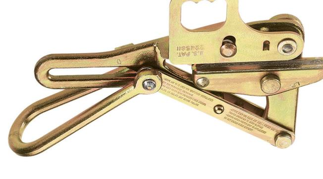
The Klein S1684-5H Chicago Grip-with Hot-Line Latch for Bare Conductors are for both bare and insulated conductors. The Klein S1684-5H Chicago Grip-with Hot-Line Latch for Bare Conductors grip may be placed on wire with hot-line stick. When stick is removed, latch closes automatically to guard against grip accidentally disengaging from wire.
