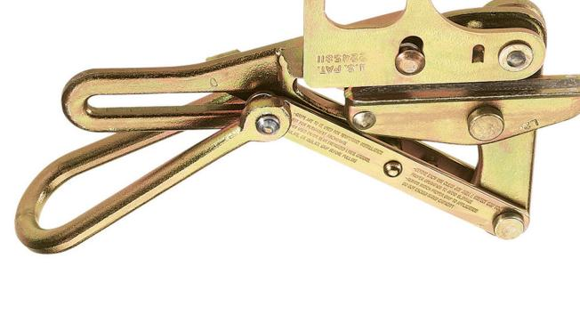
The Klein S1656-30H Chicago Grip-with Hot-Line Latch for Bare Conductors is for both bare and insulated conductors. The Klein S1656-30H Chicago Grip-with Hot-Line Latch for Bare Conductors may be placed on wire with hot-line stick. When stick is removed, latch closes automatically to guard against grip accidentally disengaging from wire.
