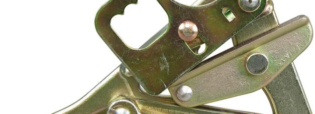
The Klein S1656-20H Chicago Grip-with Hot-Line Latch for Bare Conductors is for both bare and insulated conductors. The Klein S1656-20H Chicago Grip-with Hot-Line Latch for Bare Conductors may be placed on wire with hot-line stick. When stick is removed, latch closes automatically to guard against grip accidentally disengaging from wire.
