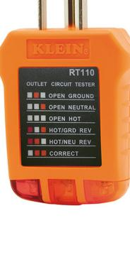
Klein Tools RT110 Receptacle Tester detects the most common wiring problems in standard receptacles. Conditions indicated: wiring correct, open ground, reverse electrical outlet, open hot, open neutral, hot/ground reversed. Conditions not indicated: quality of ground, multiple hot wires, combinations of defects, reversal of grounded and grounding conductors.
