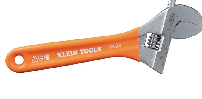
Klein Tools' 8-Inch Extra-Wide Jaw Adjustable Wrench is made of forged, heat-treated alloy steel for maximum strength and light weight. Jaws are precision-machined to ensure smooth operation. Contoured, plastic-dipped handles make them easy to grip and comfortable to use.
