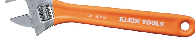
Klein Tools' 12-Inch Extra-Capacity Adjustable Wrench is made of forged, heat-treated alloy steel for maximum strength and light weight. Jaws are precision-machined to ensure smooth operation. Contoured, plastic-dipped handles make them easy to grip and comfortable to use.
