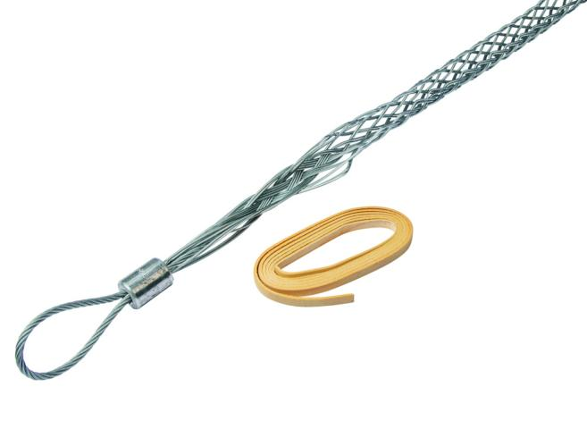
These medium-duty, standard length double-weave split mesh wire pulling grips from Klein combine strength and durability for to help linemen get the job done. Manufactured, inspected and test in the USA, these grips are made of drop-forged quality US steel. Grips are rigorously tested using the Magnaflux method and pulled to rated load to ensure the highest quality and reliability.
