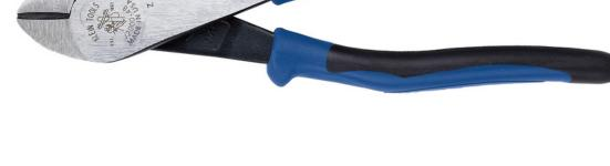
The Angled Head Diagonal Cutting Pliers from Klein Tools feature solid construction and performance for which Klein pliers are known. Short jaws and beveled cutting edges allow for close cutting of wire. They are designed with the rivet closer to the cutting edge for 36-Percent greater cutting and gripping power than other pliers designs. Klein pliers are designed and built to exceptional quality standards in a tradition that dates back to 1857.
