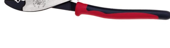
This Crimping/Cutting tool crimps insulated and non-insulated 10 to 22 AWG solderless terminals and connectors. Tapered design of the nose is great for working in confined spaces. The cutters is specially hardened for long life. The innovative dual-material Journeyman grips are more comfortable and last longer than other handles.
