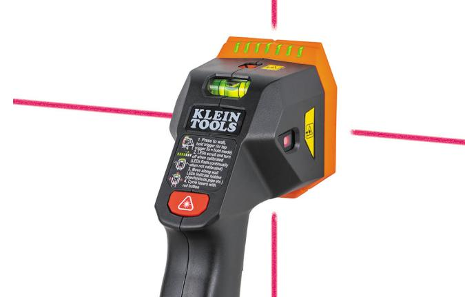
Electronic Stud Finder with Cross-Line Lasers detects hidden wood and metal studs with an auto deep scan of up to 1-1/2-Inch. The horizontal and vertical lasers can be used together or independently. Offering mutable audible alerts and bright LEDs across the top, it clearly indicates the full width of the stud. It features an ergonomic handheld grip, hold mode and withstands a 6.6-Foot (2 m) drop. Felt pads protect walls during use and bubble vial assists with alignment. Laser Class 3R; ?5mW.
