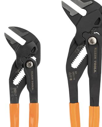
The 2-Piece Compact Plier Wrench Set includes 7-Inch (Cat. No. D5317) and 10-Inch (Cat. No. D53110) Compact Plier Wrenches with parallel jaws for a secure, damage-free grip on nuts, bolts, and workpieces. A quick-adjust button enables easy, one-handed jaw adjustment, while the high leverage ratio ensures strong grip and bending power. Laser-etched size markings make finding the right jaw opening simple and convenient.
