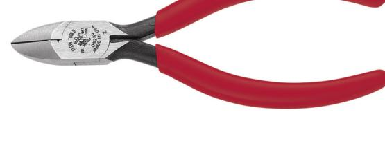
Klein Tools Diagonal Bell System Pliers feature a W notch to cleanly slit insulation and a V notch at the hinge for quick insulation crushing. The tapered nose is designed to work in confined spaces and for close tip cutting. They are manufactured from drop-forged, heat-treated steel for excellent durability.
