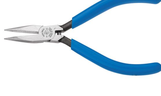
These lightweight, slim long-nose pliers feature polished inside jaws with radiused edges to prevent nicking of wire during delicate assembly work. Curved handles provide greater tool control. This pair is spring-loaded for self-opening action. Made of forged steel for maximum durability and long life.
