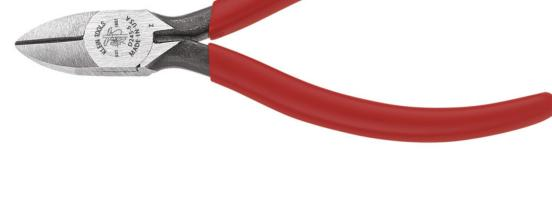
These 5-Inch Diagonal Cutting Pliers have a tapered nose to easily work in confined areas and allow close tip cutting. They come with short jaws and beveled standard cutting edges to permit close wire cuts. The pliers are forged from US-made steel and have induction hardened knives and a hot-riveted joint for a long lasting smooth action.
