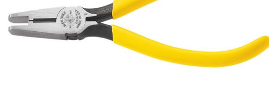
These Klein Tools Connector Crimping Pliers are designed to crimp and seat UG, UR and UY connectors. They have a hot-riveted spring assisted joint for smooth, self opening action. And they have induction hardened side cutting knives and curved handles for improved performance and durability.
