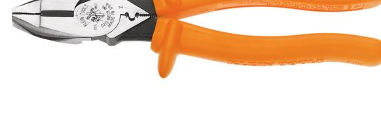
These Klein Tools 9-Inch Insulated Side-Cutting Crimping Pliers offer protection against electric shock up to 1000 volts. The pliers are individually tested to exceed the IEC 60900 and ASTM F1505 standards, for insulated tools, and clearly marked with the official 1000-volt rating symbol. The pliers offer maximum strength with their forged-steel construction and a crimping die helps provide increased leverage.
