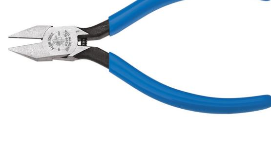
These Klein Tools 5-Inch Electronics Pliers have a narrow jaw and hinge with a sharp, pointed nose for precise tip cutting and trimming of printed circuit boards. Made of US-made steel and induction hardened for long life. Spring assisted, hot-riveted joint for a smooth action and no wobble handle. The handles are plastic dipped for comfort and ease of identification.
