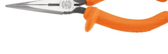
Klein Tools Insulated Long Nose Side-Cutting pliers are 1000V rated for safety on the job. The long nose is designed for grabbing and looping wire. Dual layer, orange-over-white insulation provides a warning sign that insulation may be compromised. The molded insulation meets or exceeds ASTM F1505-16 and IEC 60900:2012 standards for insulated tools. Cutting knives are induction hardened for long life.
