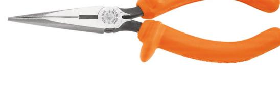
Klein Tools Insulated Long Nose Side-Cutting pliers are 1000V rated for safety on the job. The long nose is designed for grabbing and looping wire. Dual layer, orange-over-white insulation provides a warning sign that insulation may be compromised. The molded insulation meets or exceeds ASTM F1505-16 and IEC 60900:2012 standards for insulated tools. Cutting knives are induction hardened for long life.
