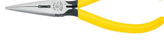
These Long-Nose, Side-Cutters also cleanly strip 19-22 AWG wire found in switchboard work. The cutting knives are induction hardened for maximum life. Made of forged steel for durability with a long nose for grabbing and looping wire.
