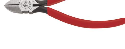
These Klein Tools Spring-Loaded Diagonal Cutters are designed to work easily in confined areas thanks to their short jaws and spring assisted hot riveted joint giving it a smooth action. The pliers are made of US steel with induction hardened knives. The handles are plastic dipped for comfort and ease of identification.
