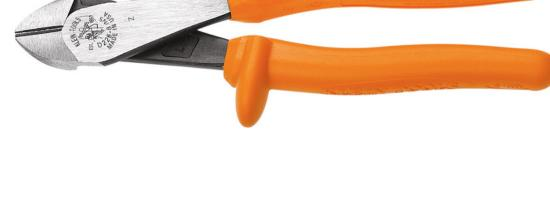
These 8-Inch Klein Tools Insulated Heavy-Duty Diagonal-Cutting Pliers have durable molded insulation that is flame retardant, impact resistant and clearly marked with 1000-volt rating. The knives are heavy duty induction hardened steel that can cut ACSR, screws, nails, and most hardened wire. Their high-leverage design allows for them to have 36-percent greater cutting power than other similar plier designs.
