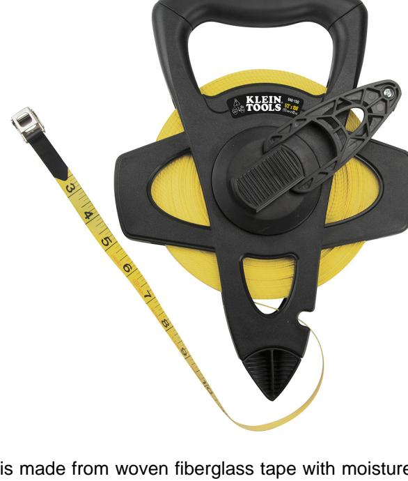
Klein Tools 150-Foot (45.72 m) Tape Measure is made from woven fiberglass tape with moisture-proof coating of polyvinyl chloride assures durability and protects against oil or chemicals. All metal parts are nickel plated for protection against rust. Tape line is graduated in feet and inches to 8ths.
