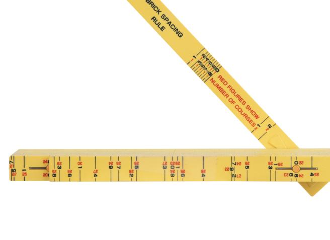
Klein Tools' 6-Foot Brick Fiberglass Folding Ruler is constructed of tough nylon, reinforced with glass fibers for added durability, and resistance to weather, abrasion, and most chemicals. Inch measurements are marked on both edges of the outside faces of the rulers, graduated to 1/16-Inch (1.6 mm). Standard brick scale measurements are marked on the inside faces of the rulers. Graduations are engraved on both sides with brick scale units on the other side for versatility.
