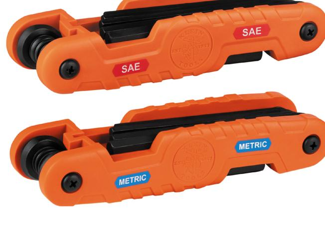
Klein Tools 2-Piece Pro Folding Hex Key Set features 21-Keys including SAE and metric Sizes. This set combines the 11 most common SAE sizes and 10 common metric sizes all in one set to tackle any job. The hex ends are square-cut for a secure full-depth fit and maximum contact with the hex socket to prevent slippage and stripping of the socket.
