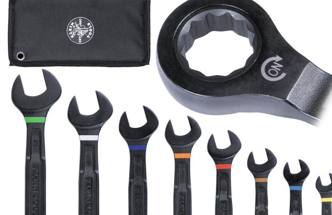
The Klein Tools Ratcheting Combination Set contains eight SAE wrenches with color coded size markings to easily identify each tool. These wrenches are made from cold-forged steel alloy precision machining finish and black phosphate coating for long-lasting rust prevention. The 90-tooth ratchet mechanism minimizes the return angle for maximum access.
