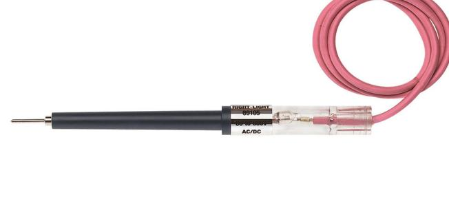
Tests circuits rated from 80 to 600 volts AC/DC. The high-impact, sealed 5-11/16" (144 mm) probes on long 24" (610 mm) leads are convenient for testing motors, fuses, relays, switches, etc. A professional grade electrical tester with the quality you expect from Klein Tools.
