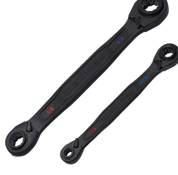
The Klein Tools 4-in-1 Ratcheting Wrench Set is a versatile box wrench set featuring two 12-point socket wrenches with eight SAE hex sizes, including 1/4, 5/16, 3/8, 7/16, 1/2, 9/16, 5/8, and 3/4-Inch. Features 90-tooth ratchet mechanism minimizing arc swing for access in tight spaces and a pass-through design accommodates longer threads. The reversing switches enable quick direction changes and ergonomic handles provide optimized comfort during extended use or repetitive tasks.
