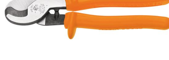
Use the Klein Tools Insulated Cable Cutter when cutting cable where there is a risk of electrical shock. This cable cutter offers protection up to 1000 volts and features a one-handed shearing design for easy operation. It is individually tested to exceed the IEC 60900 and ASTM F1505 standards, for insulated tools, and clearly marked with the official 1000-volt rating symbol.
