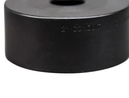
Klein 2.416 Knockout Die allows you to easily punch holes for 2-Inch EMT conduit. Has a maximum capacity of 10 gauge mild steel. Cuts aluminum, fiberglass and plastic as well.
