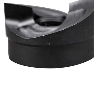
Easily punch holes for 1-1/2-Inch EMT conduit. Has a maximum capacity of 10 gauge mild steel. Cuts aluminum, fiberglass and plastic as well. Optimized design reduces wrench effort. Slugs are split inside for easy removal.
