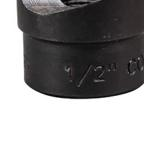
The 7/8-Inch Knockout Punch easily punches holes for 1/2-Inch EMT conduit. The optimized design reduces wrench effort. Slugs are split inside for easy removal. Cuts aluminum, fiberglass and plastic as well.
